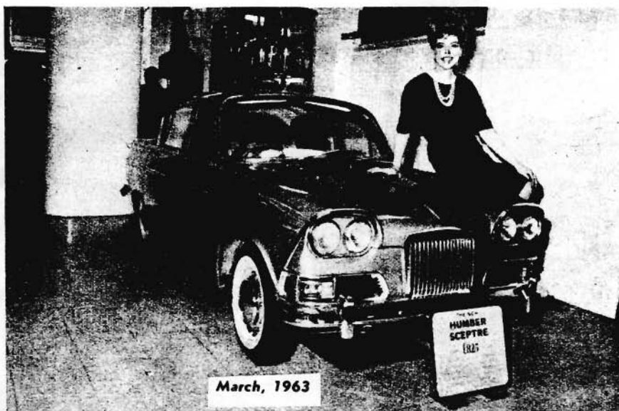
The new Humber Sceptre — latest in the Humber range on show in London. The four cylinder 1592 c.c. engine develops 85.5 bhp at 5200 revolutions a minute with maximum speeds of about 28 mph in first, 45 in second, 68 in third and 85 in top.
