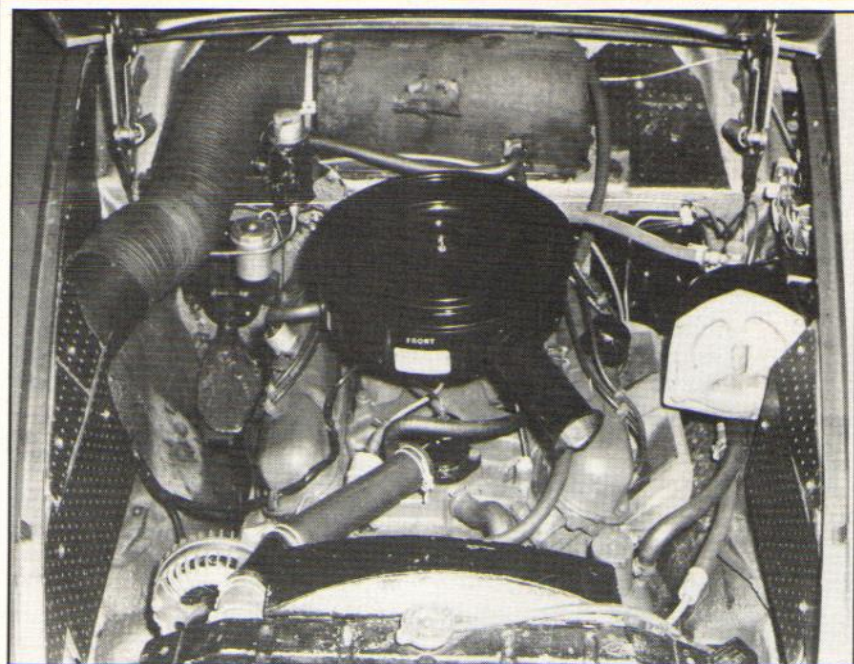
There was sufficient space under the bonnet of the Snipe for a V8 to fit without major body modifications
